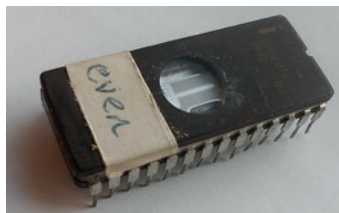
Figure 2.26 EPROM device from the 1980s. The silicon die is visible through the top window
